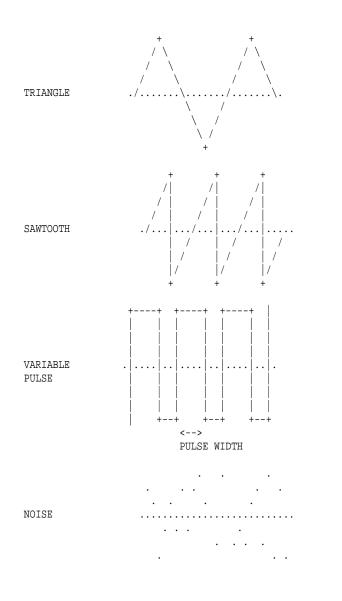
Figure 7-3. Sound Waveform Types
