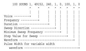
Line 100 starts the sweep frequency at 49152 and decrements the sweep by 100 in the downward direction, until it reaches the minimum sweep frequency at 0. Voice 1, using the sawtooth waveform (#1), plays each SOUND for four seconds (240 \* 1/60 s). Line 100 sounds like a bomb dropping, as in may "shoot 'em up" arcade games.
